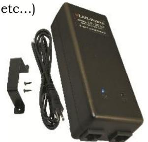
**Verifying Contents of Package** - Unpack the PoE Injector and verify that you have all of the following items: Single Port Power over Ethernet Injector, IEC320 inlet 2Pin-C8 Mains Power Cord and Mounting Bracket with Screws
